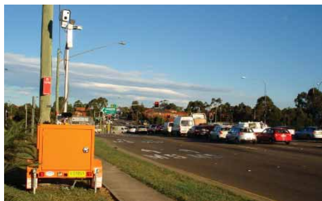
The mobile engine brake noise camera trailer system at work.
