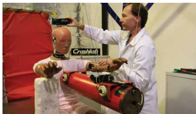
RTA staff member Andrew Stanley preparing a crash test dummy in a process referred to as 'dummy calibration'.
